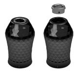
7. Turn the grip adapter 90° counterclockwise and remove it from the grip.
