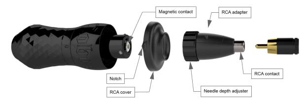
The RCA adapter is swivelling to prevent the RCA cable from twisting during operation and when the needle depth is adjusted.
