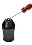
8. Tighten the screw with the 0.9 Hex key (red) from the *Precision tool kit No. 90*. Make sure the key engages in the screw properly before tightening so the screw is not damaged. Tighten medium hard and make sure you don't bend to the side which can damage the key or screw.
