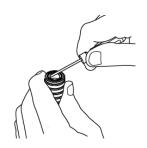
6. Loosen the grip adapter screw with the 0.9 Hex key from the *Precision tool kit No. 90*.
