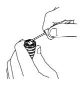
8. Tighten the screw with the 0.9 Hex key (red) from the *Precision tool kit No. 90*. Make sure the key engages in the screw properly before tightening so the screw is not damaged. Tighten medium hard and make sure you don't bend to the side which can damage the key or screw.
