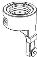
3. Leave the Magnet holder screw in the Magnet holder to prevent the screw from disappearing. Keep the magnet in a plastic bag to keep free from dirt.
