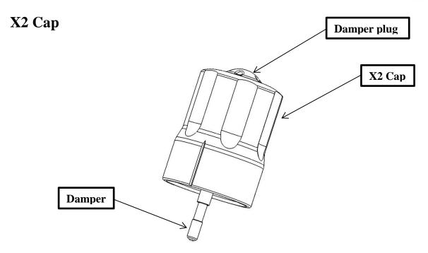
The new X2 cap has a built in Damper that prevents clatter and noise when the give adjustment is used.
