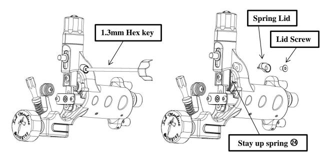
To take advantage of the give function when using cartridges the Inner piston spring should be replaced. If the give function is not required just adjust the give to the bottom position (hardest setting).
