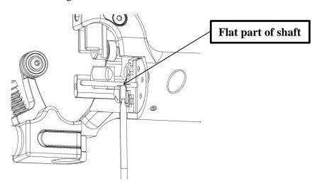
8. Put the **Rod assembly**  and the **Shaft support** in place and tighten the **Shaft support screws** . The **Shaft support** must be oriented with the clearance groove downwards or the **Rod assembly** won't fit properly.
