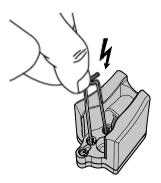
Make a hard reset by short circuiting the battery. Use a metal clip or similar to connect the
